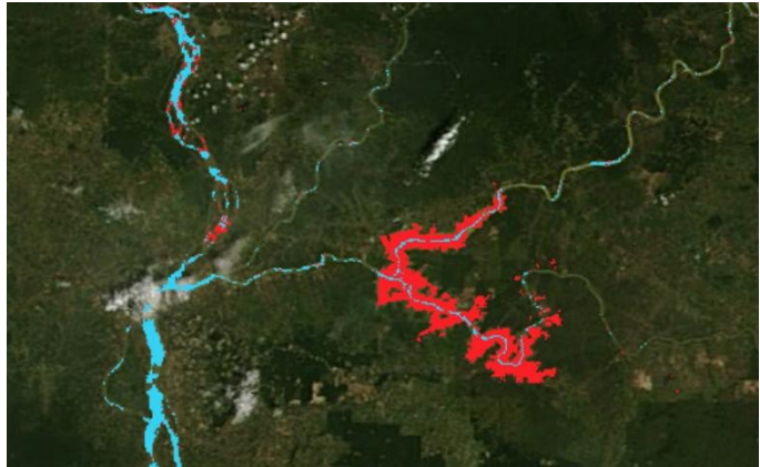
Figure 14: Example: New reservoir misidentified as flood. Lower Sesan II dam in Cambodia, 2-Day product, 11 Nov 2022, Worldview display.
